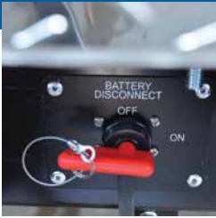
12 Volt Disconnect provides for easy power shut-off
