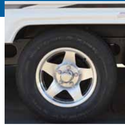
Aluminum Wheels look good, are lighter and dissipate heat better
